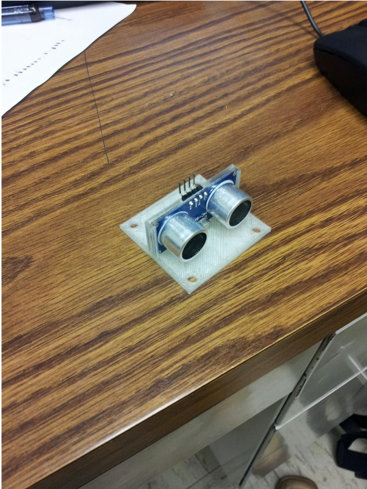
Figure 11: All of the sensitive electronics on the back of the board are covered by the plastic so that only connectors are exposed.
