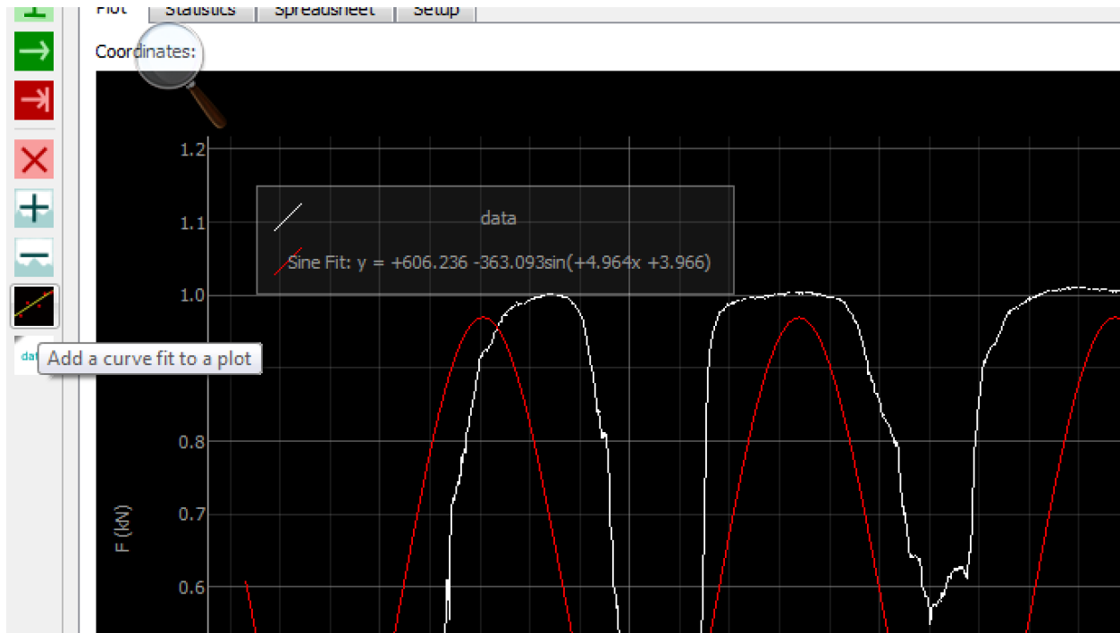
Figure 7: In case the user forgets what the icons do, all they have to do is hover the mouse over the icon for a few seconds and the functionality will be displayed – as seen in this zoomed in view of the screen.
