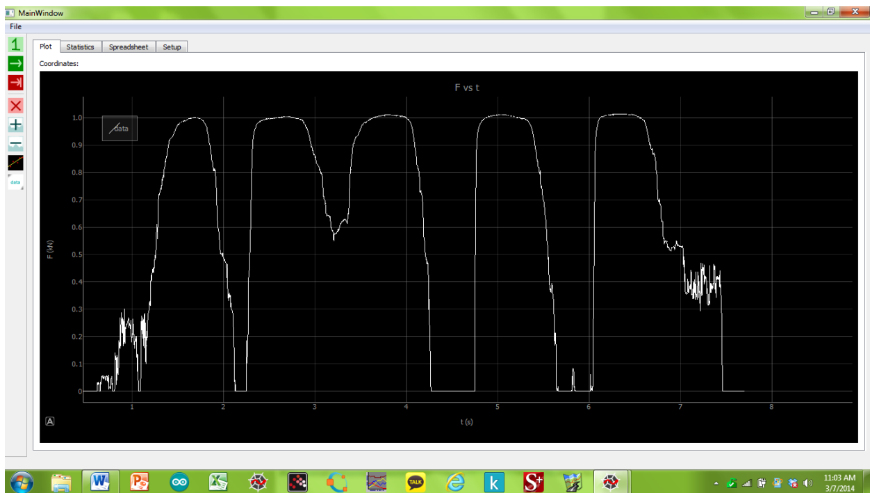
Figure 1: A view of plotted data that I acquired using my finger to press periodically on a force sensor.
