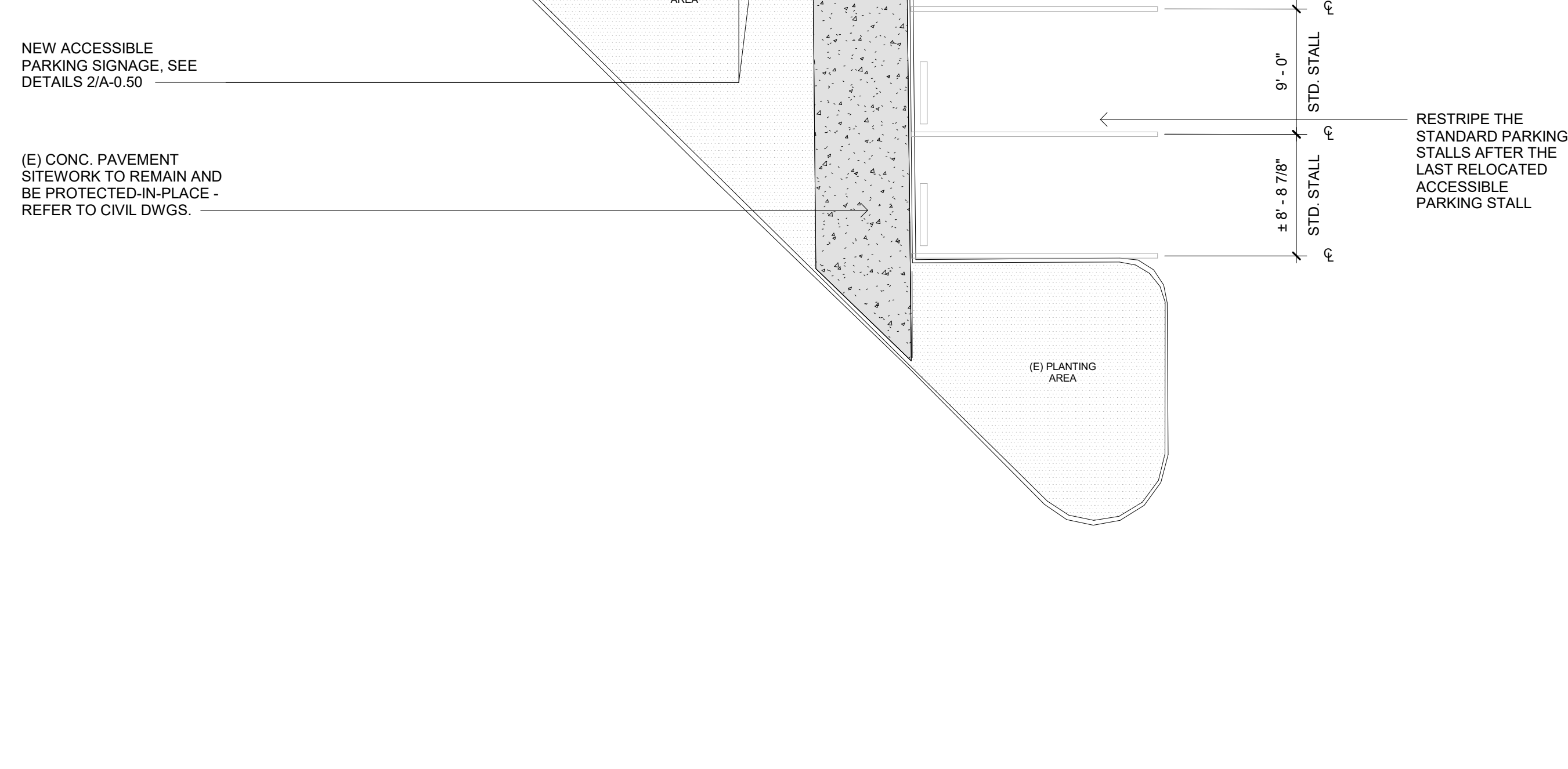
ENLARGED PLAN OF NEW ACCESSIBLE STALLS 1/8" = 1'-0" 6
