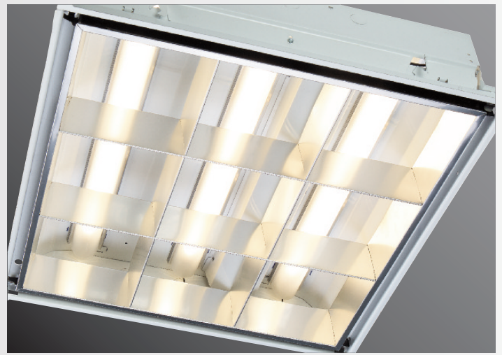
Three 2' strips in a 2x2 parabolic troffer utilizing a 22W driver with diffusers. This Stripit Kit ® replaced two F40 4 pin U-Tube lamps (40W ea). Lights levels increased by 19% with a 72% reduction in energy.
