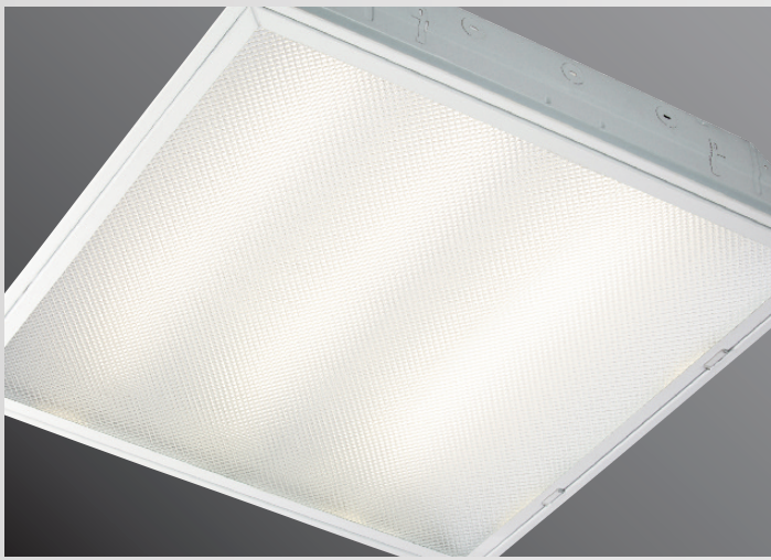
Three 2' strips in a 2x2 prismatic troffer utilizing an 18W driver without diffusers. This Stripit Kit ® replaced two 32 watt U bend fluorescent tubes. Lights levels increased by 23% while reducing energy consumption by 72%.
